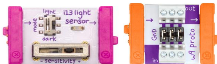
Fig. 6. Receiver components: Light sensor and proto bits.
