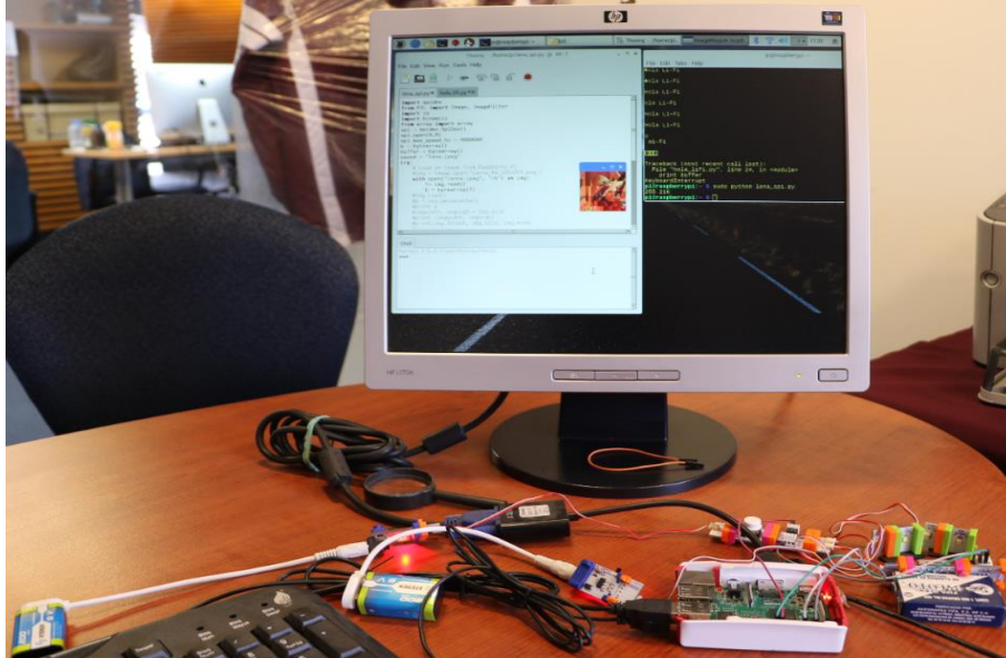
Fig. 11. Setup for the transmission and reception of text and an image using VLC.
