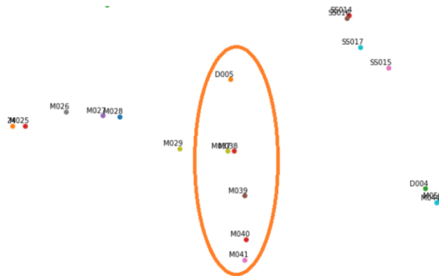
Fig. 4. Extract from the t-SNE plot of the activity of sensors from the CASAS Kyoto-20 dataset [11], using 600 seconds as the interval and time decay factor weight x^t for x=0.9 and t being the time gap in multiples of 15 sec, showing the contextual proximity of the motion sensors close to the toilet (M038 to M041) and door sensor D005.
